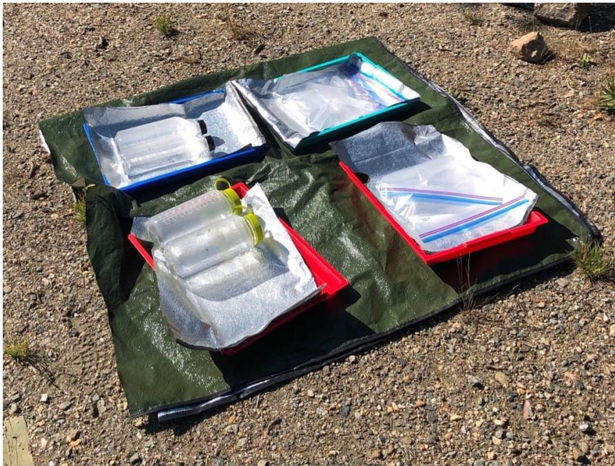
Caption: Experimental set up with Nalgene bottles, plastic water bottles, and a plastic bag placed on a reflective tarp exposed to the sunlight during a lower-altitude trial (Credit: Kylie Van Hoesen, MD).
