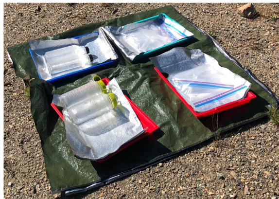
Figure 1. Experimental setup with Nalgene bottles, plastic water bottles, and a plastic bag placed on a reflective tarp and exposed to the sun during a lower-altitude trial.
